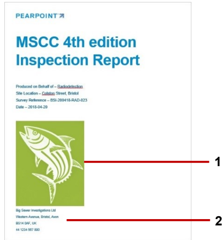
Fig. 5-23: Example title page for MSCC4 exported survey report (Microsoft Word format only). 1 Your company logo. 2 Your company name, address and phone number
