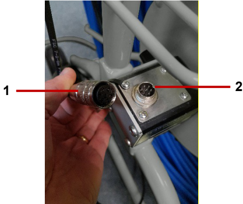
Fig. 4-23: Link cable (1) connects to the pushrod reel (2)
