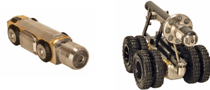
Fig. 3-9: P354 crawler with Forward View camera installed and P356 crawler with pan, tilt and zoom camera, large elevator and lighthouse installed.
