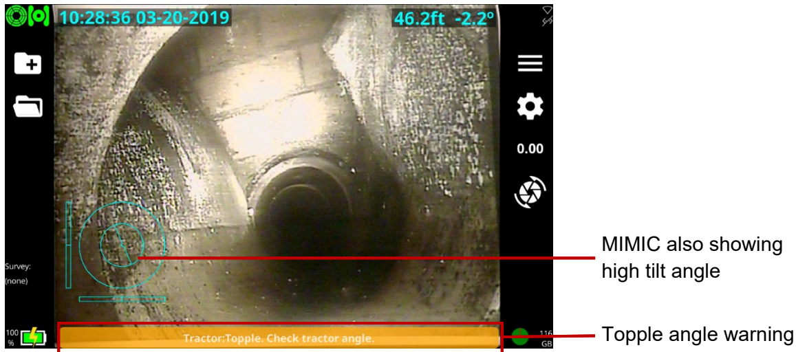
Fig. 6-14 Topple warning shows at the bottom of the screen. Note that the MIMIC also shows a high tilt angle.
