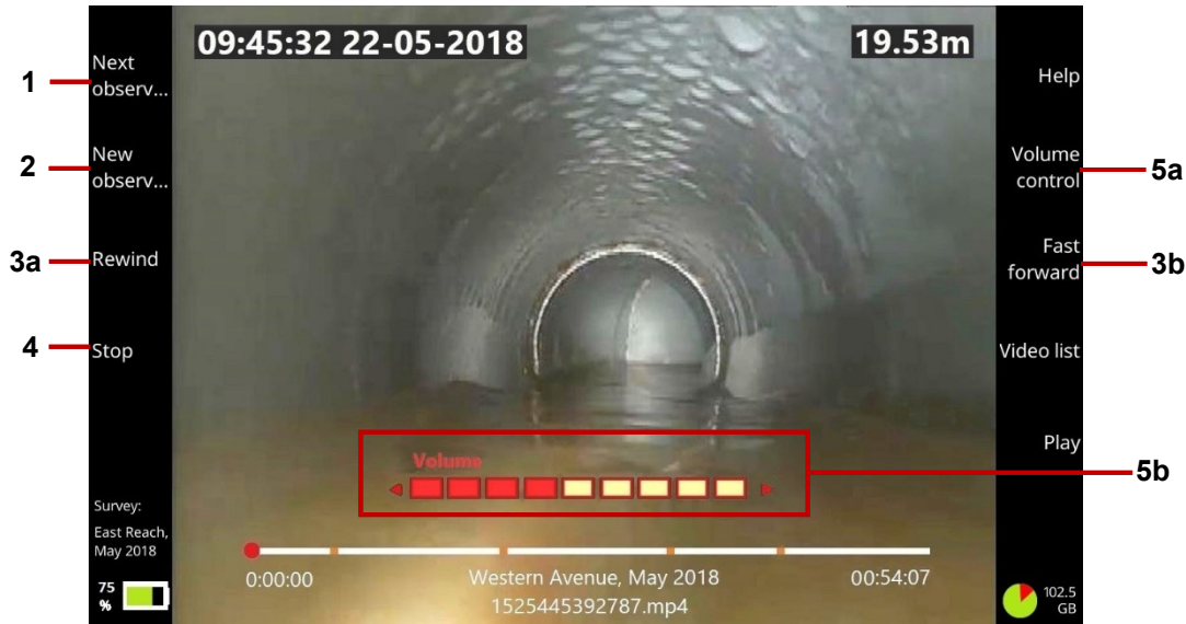
Fig. 6-31: Video playback screen. 1 Next observation button. 2 New observation button. 3a, 3b Rewind and Fast Forward buttons. 4 Stop button. 5a Volume Control button. 5b Volume level Use the ⇐ ⇨ arrow keys to adjust the volume.
